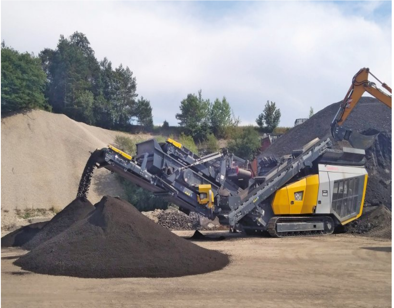
Keestrack R3e mobile impact crusher for aggregates and recycling applications with advanced innovative diesel/electric drive with plug-in functionality
