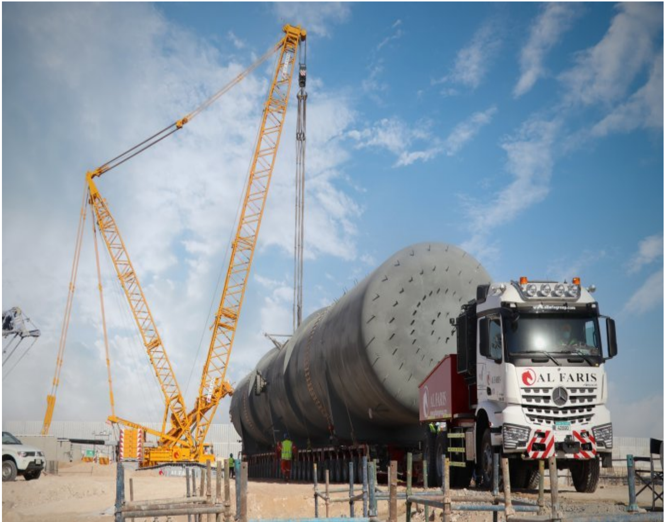
Safe journey on Goldhofer THP/SL heavy-duty modules with 30 axle lines: from Jebel Ali Port to the offloading point at Mohammed bin Rashid Al Maktoum Solar Park.
