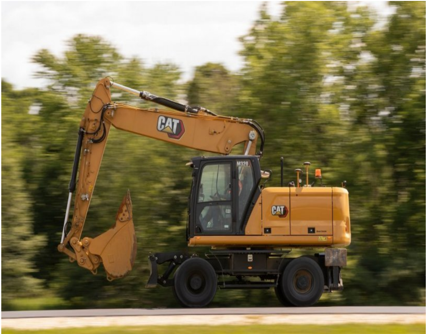
new Cat® M320 wheeled excavator
