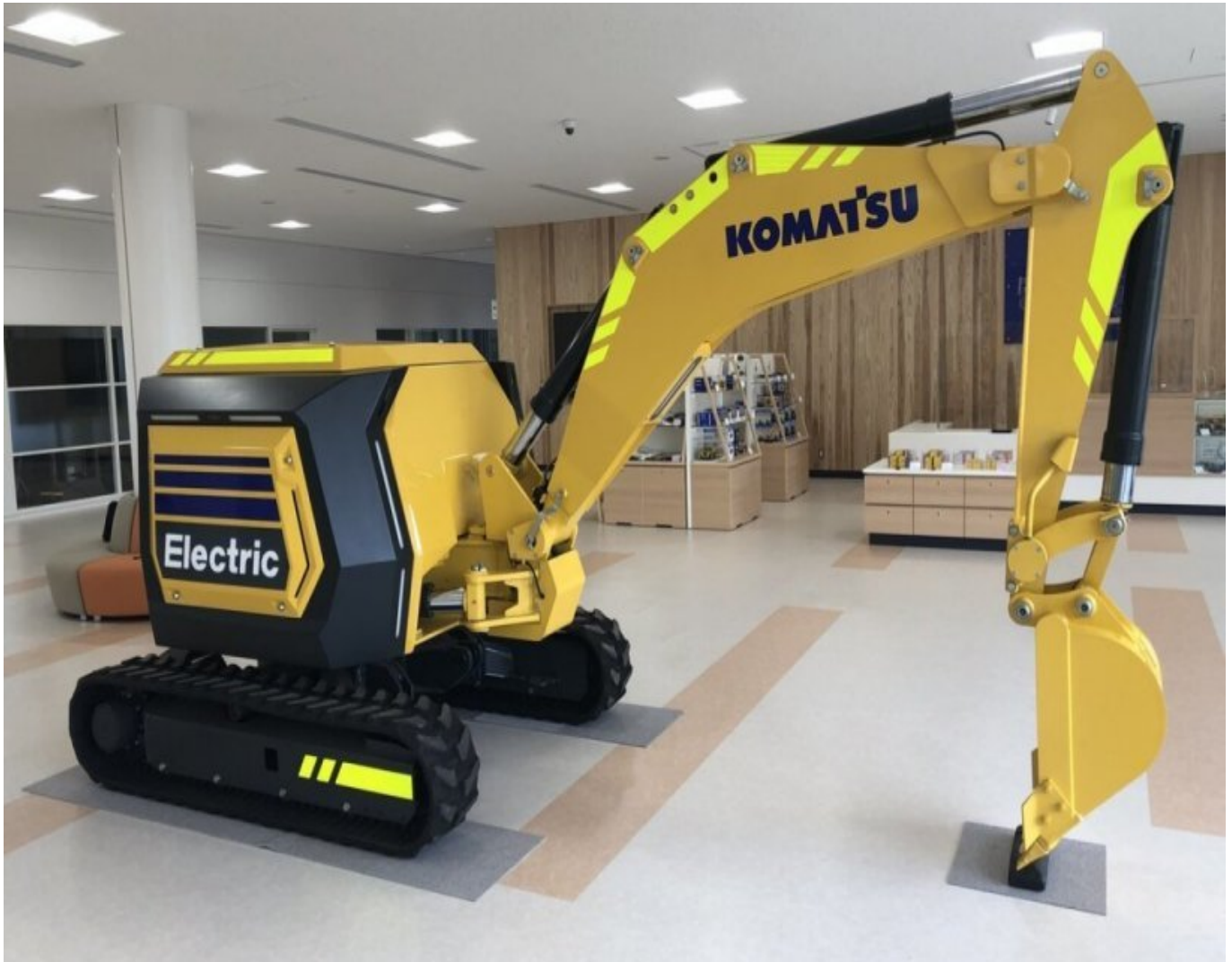
Fully electric mini excavator as the next generation concept machine for the future
