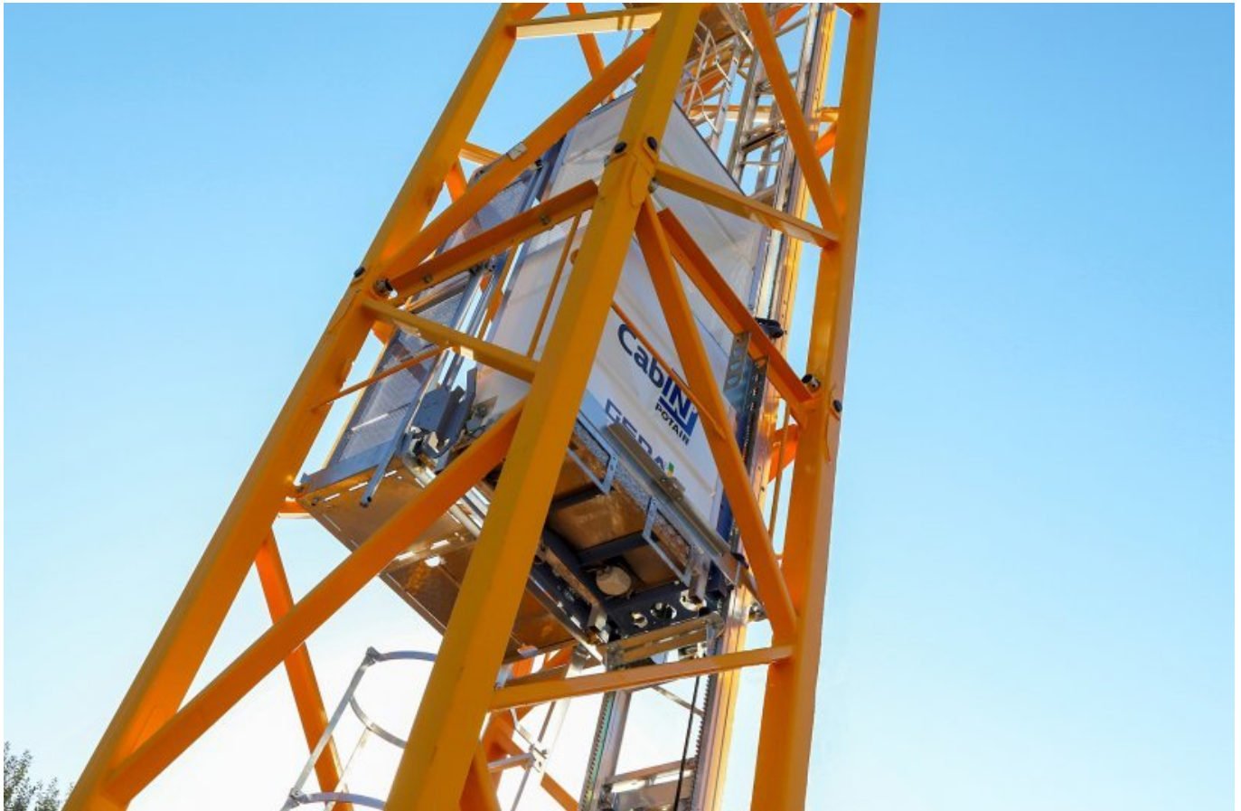
new Cab-IN internal mast elevator IMAGE SOURCE: The Manitowoc Company, Inc.
