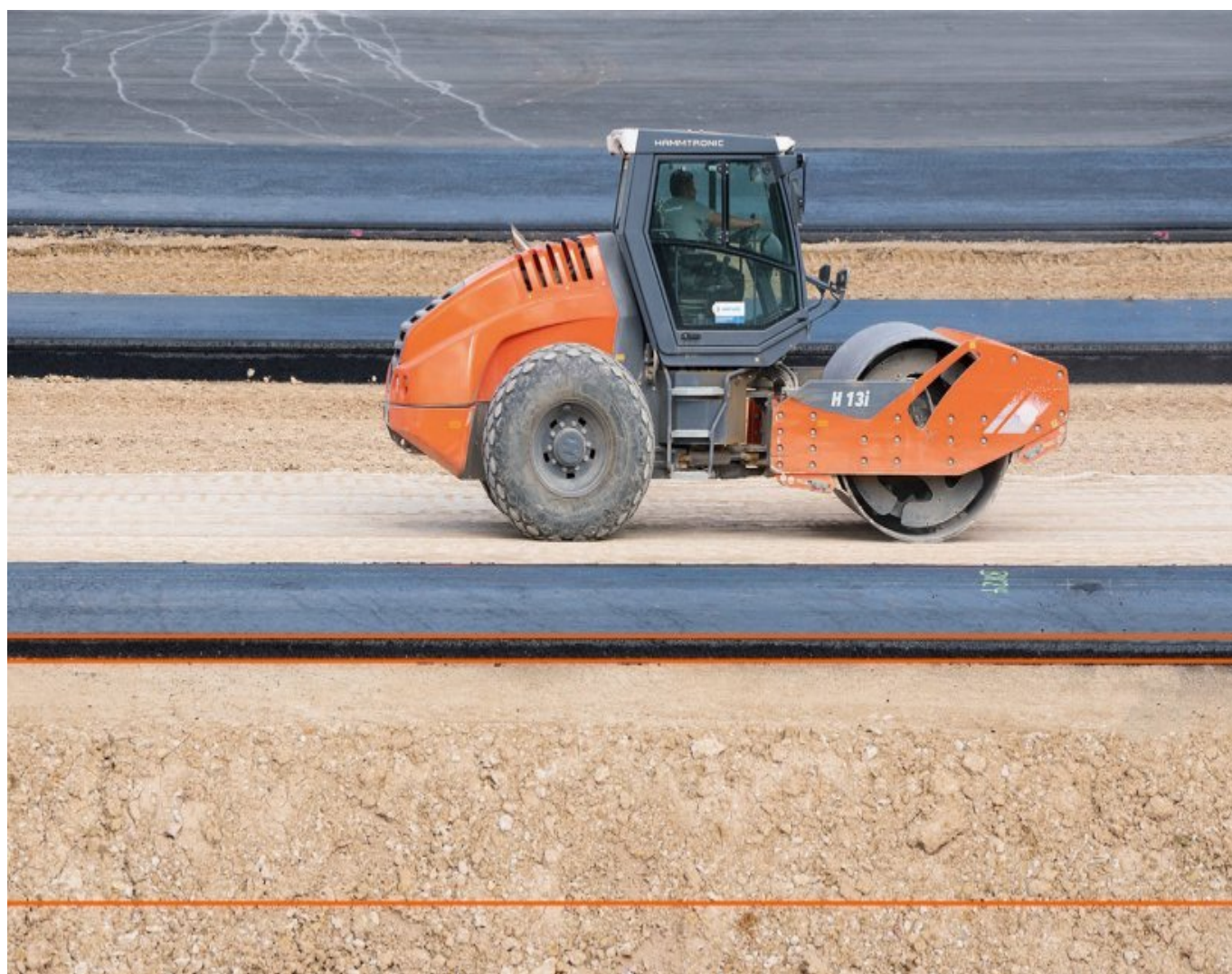
Hamm compactor with a smooth drum H 13i
