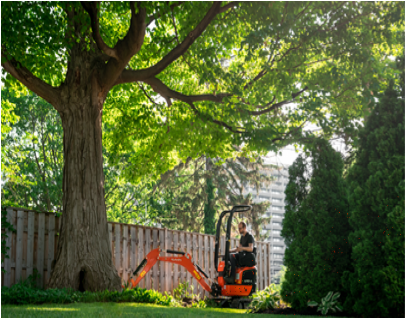
Kubota U10-5 features the so called minimal tail swing
