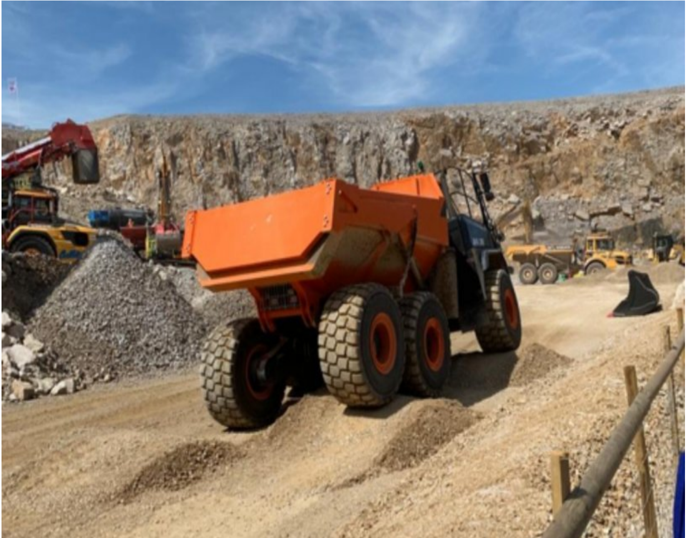
Humps demonstrating continuous 6-wheel ground contact of Doosan
