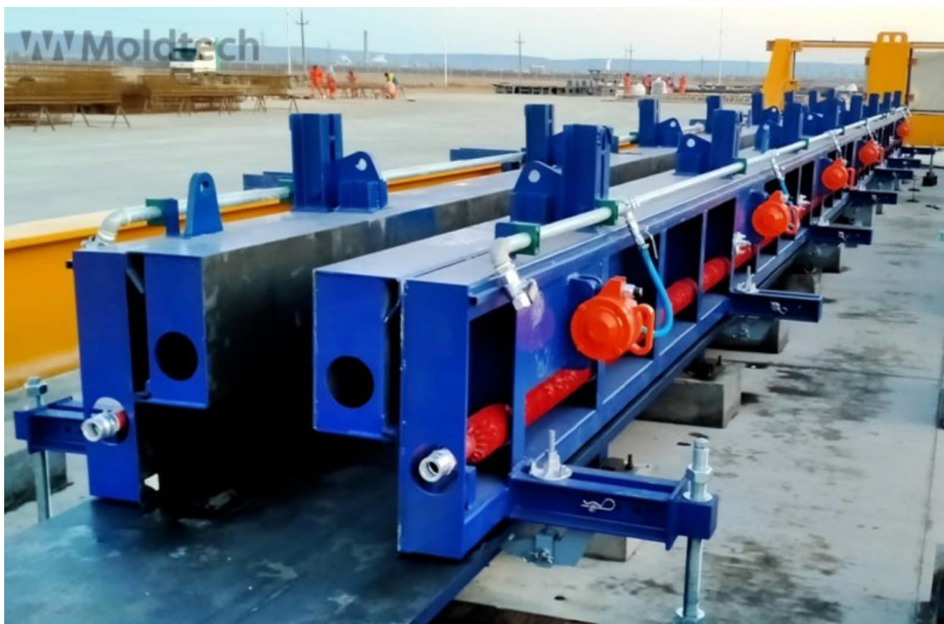
Mould for beams
