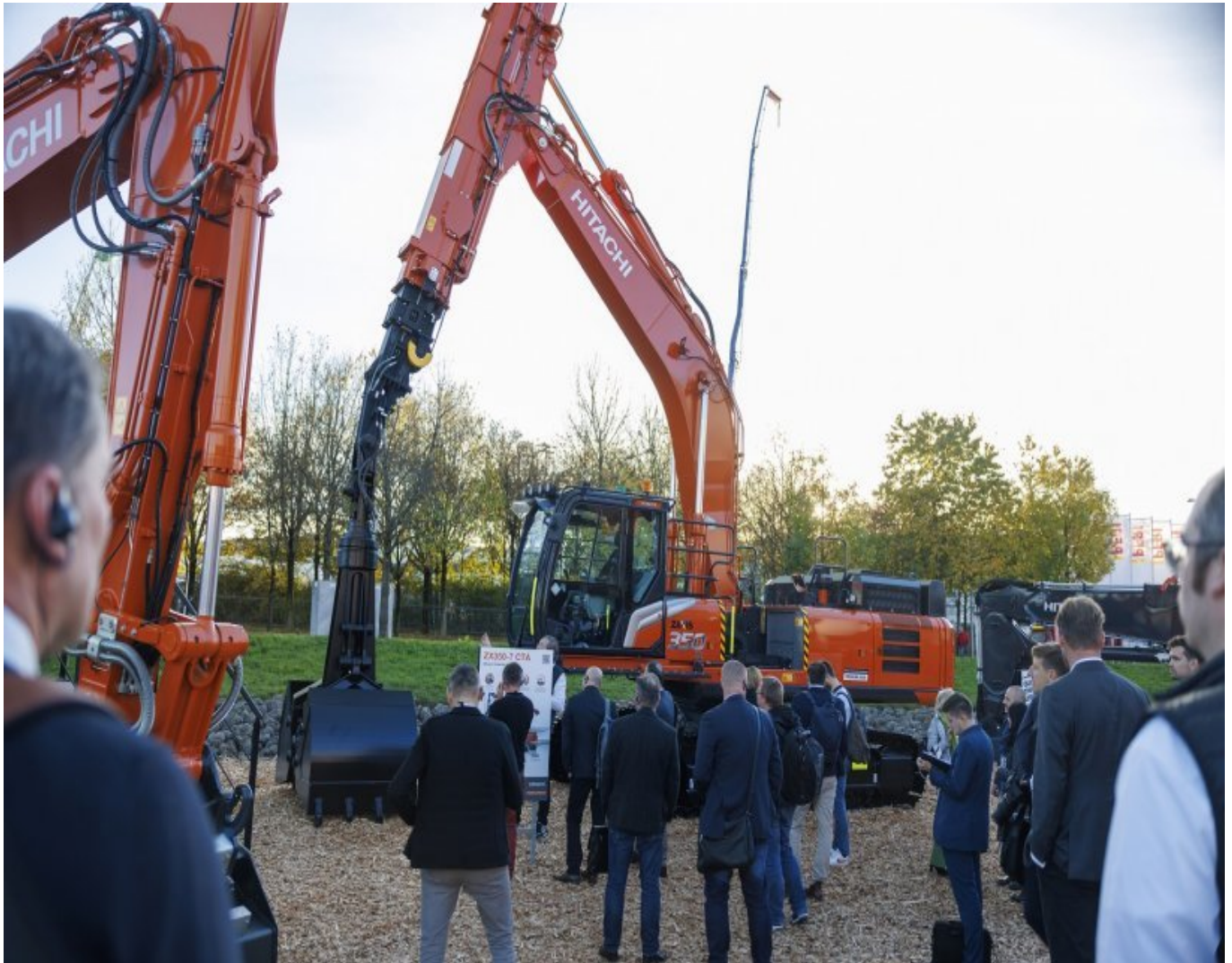
Hitachi ZX350LC-7 excavator with clamshell telescopic arm
