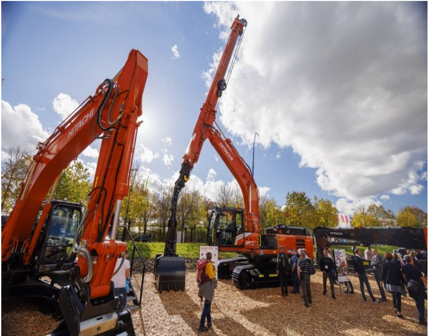
Hitachi ZX350LC-7 excavator with clamshell telescopic arm
