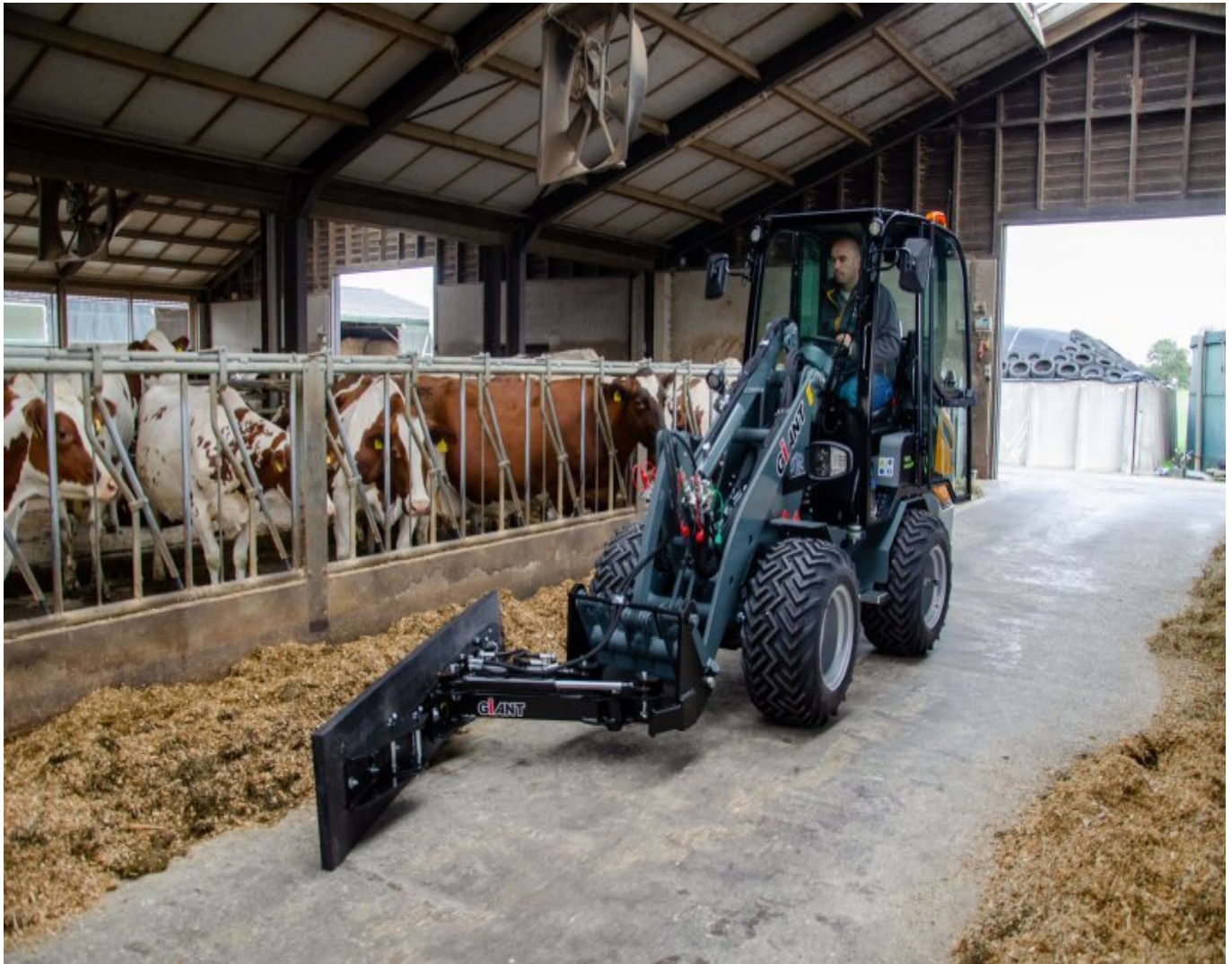
G2200E with hydraulic feed and manure scraper
