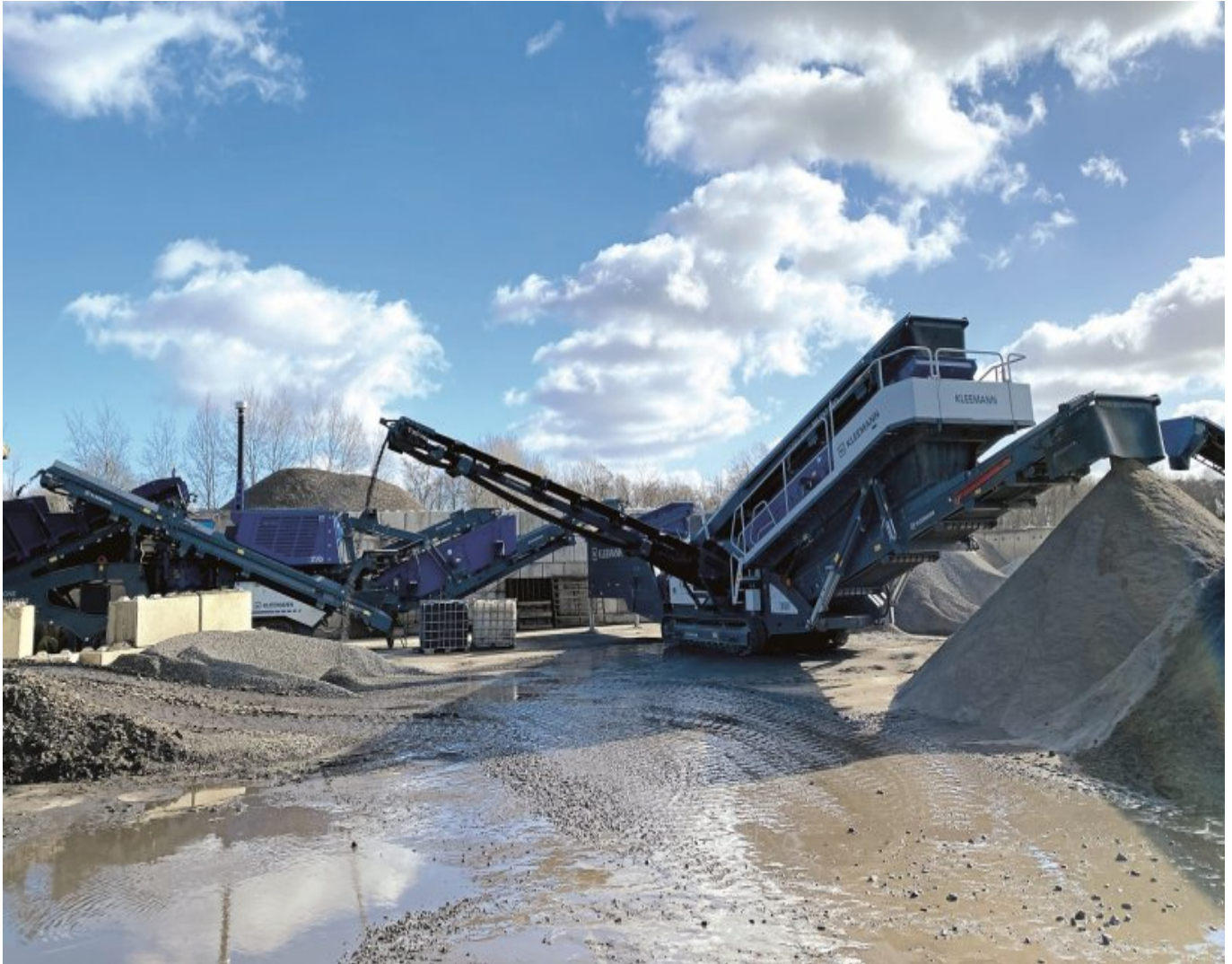
The MCO 90i EVO2 and MS 953 EVO are connected with one another by line coupling.
