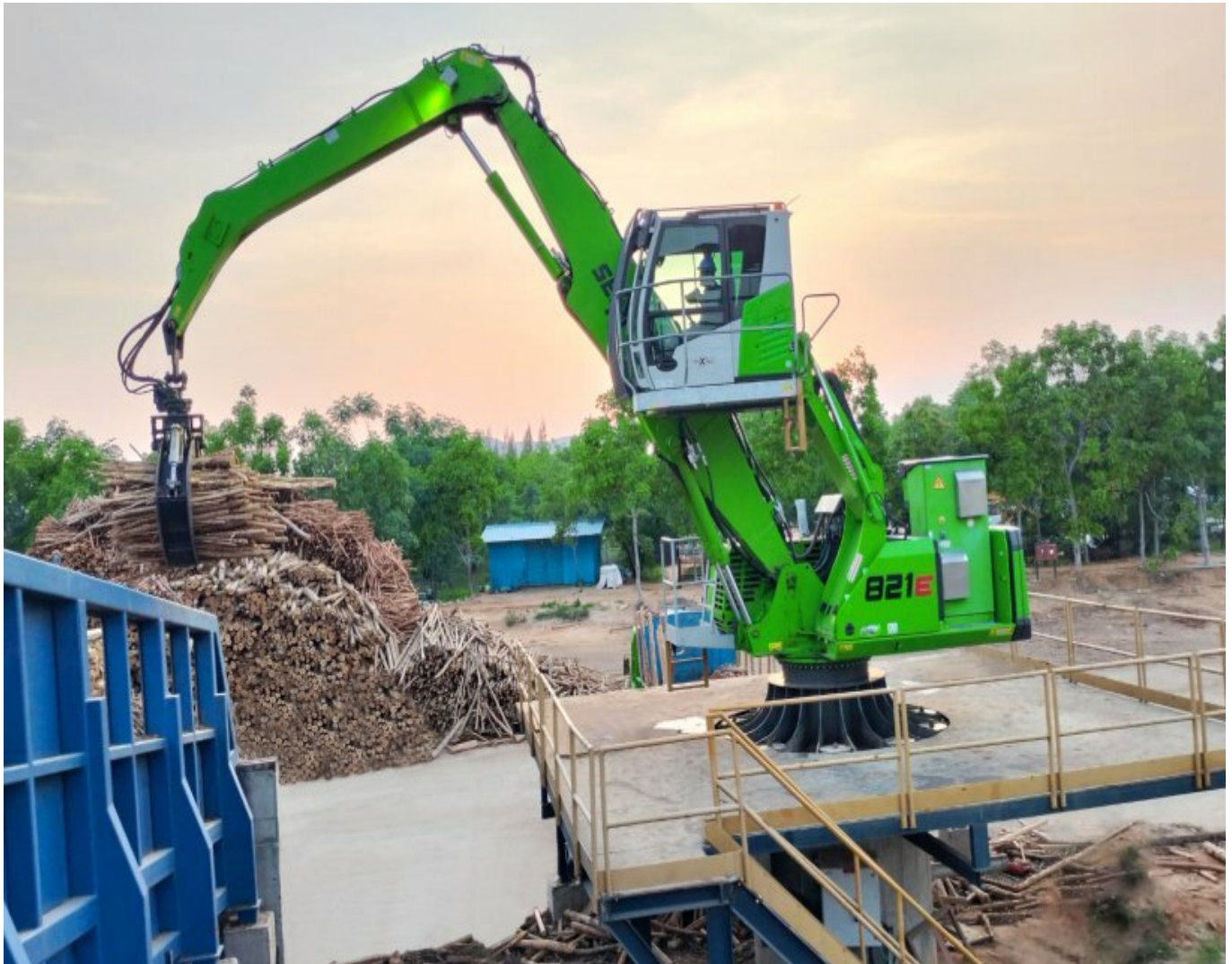
Efficient timber handling: The stationary 821 E Electro proves its high handling capacity when feeding the conveyor belt with logs.
