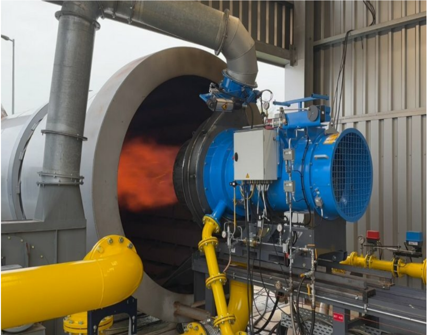
The prototype on the burner test bed at the Benninghoven factory. The new burner generation enables the use of four different fuels at the same time.
