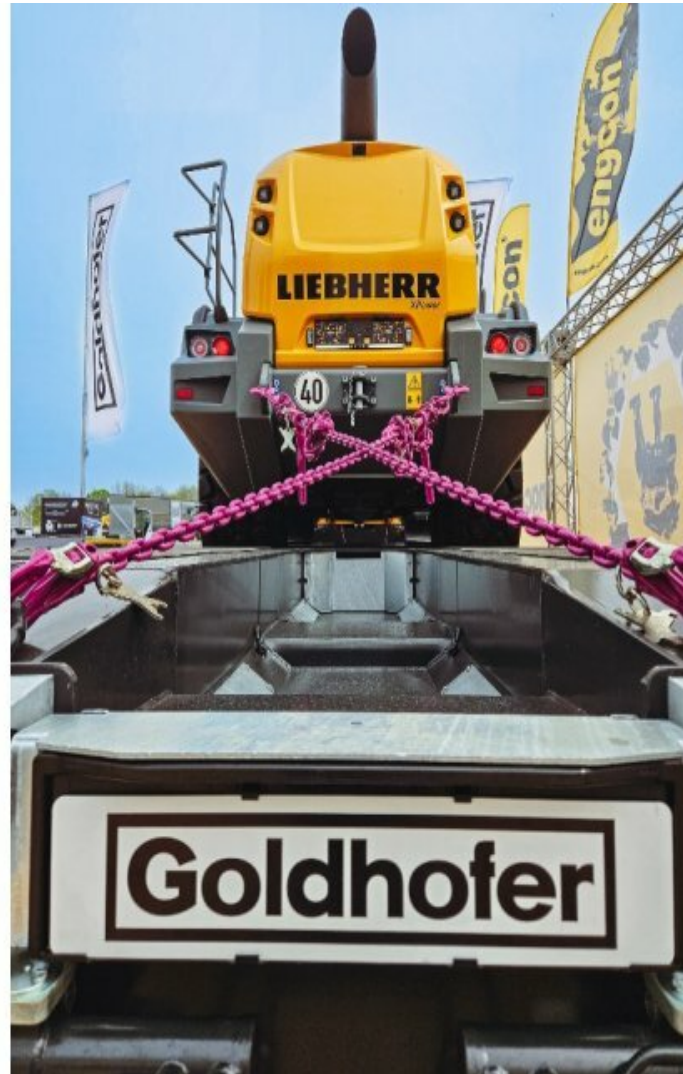
A Liebherr L550 on the versatile Goldhofer STZ-L4 with wheel recesses.
