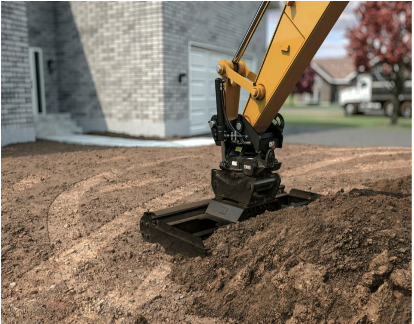
Pairing a grading beam with a tiltrotator's 360° bidirectional and 45° left and right rotation for dynamic grading.
