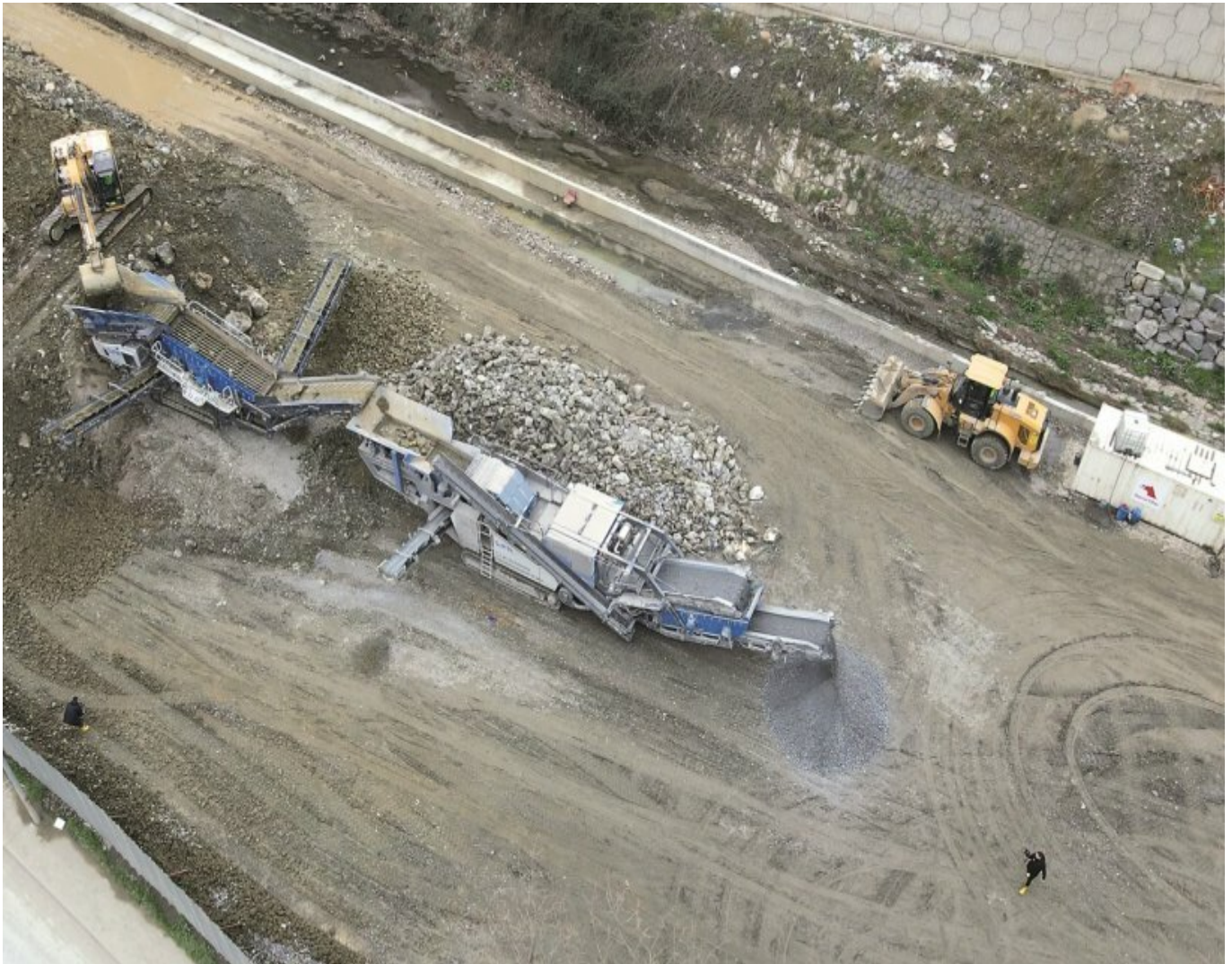
Plant train consisting of MOBIREX MR 130i EVO2 and MOBISCREEN MSS 802i EVO during material processing for concrete production and road substructures.
