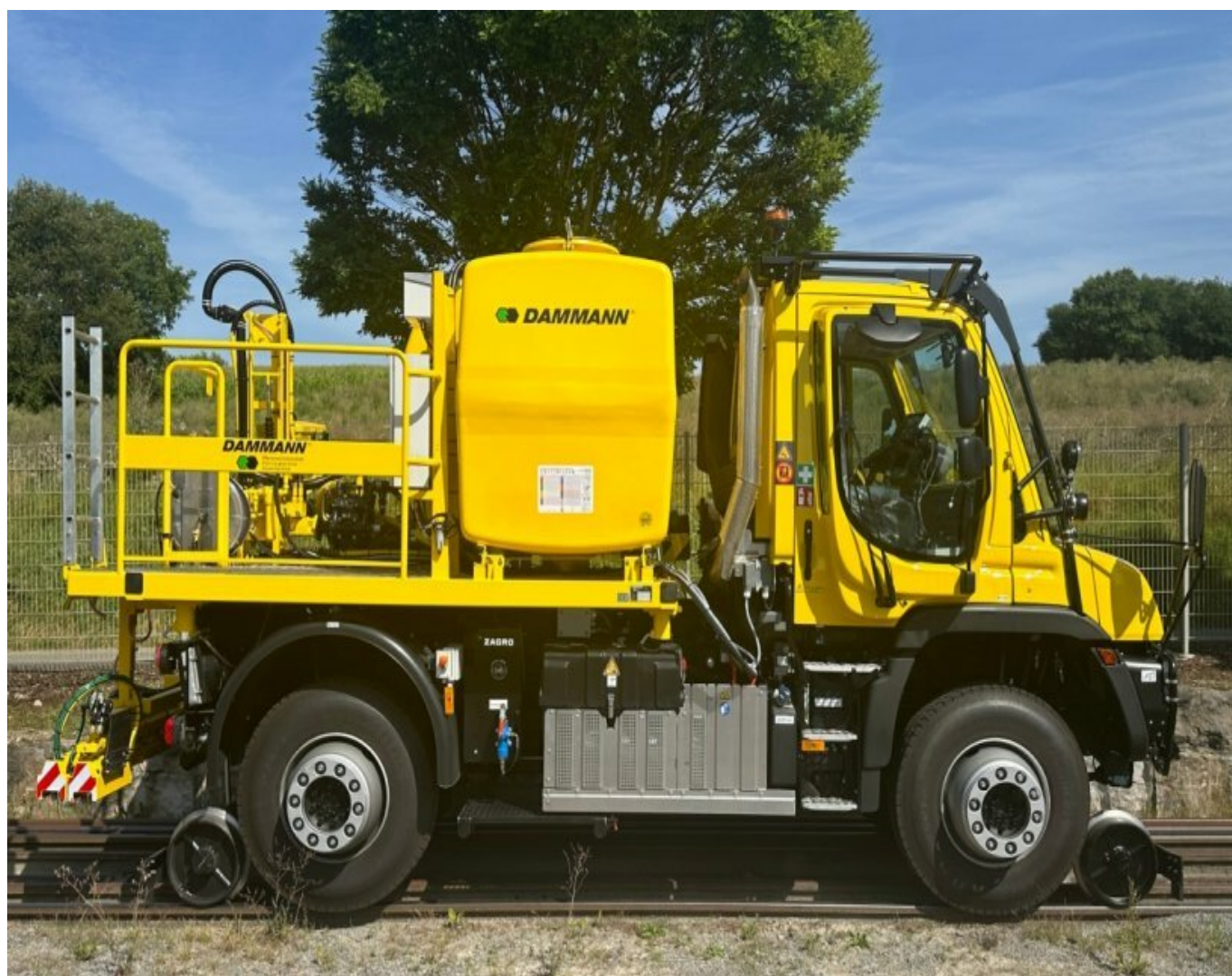
ZAGRO equips the Unimog for maneuvering/shunting tasks and track maintenance
