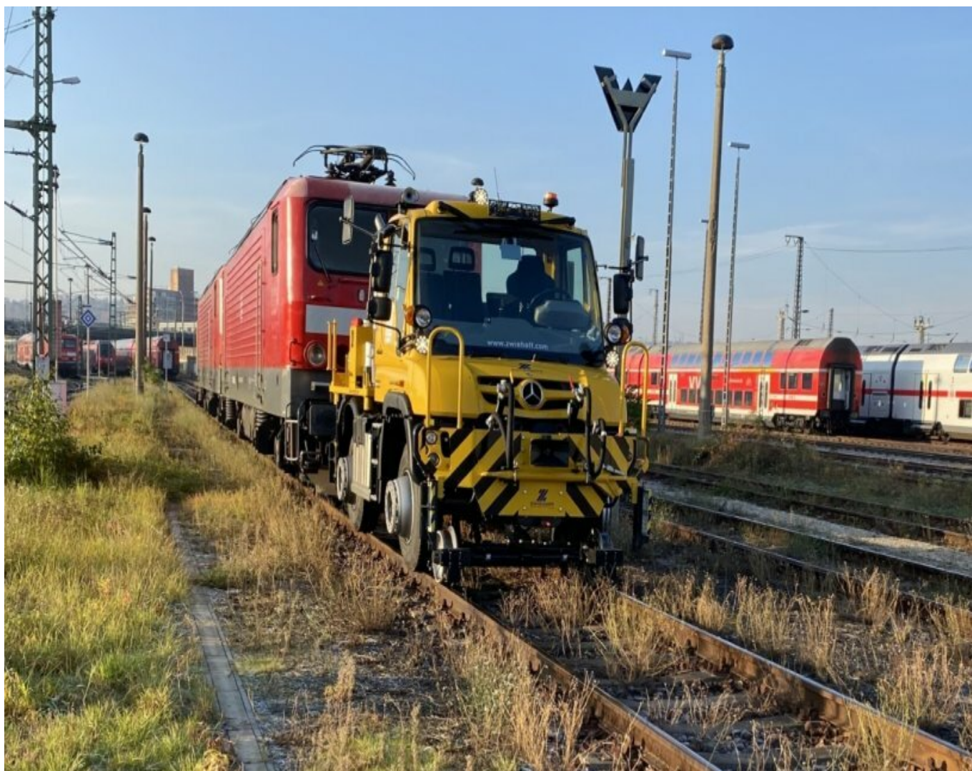
Radio-controlled Unimog shunting vehicle from Zwiehoff
