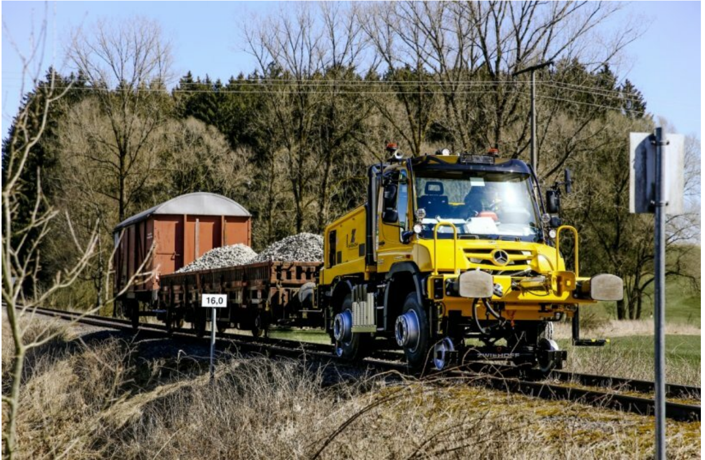
Radio-controlled Unimog shunting vehicle from Zwiehoff
