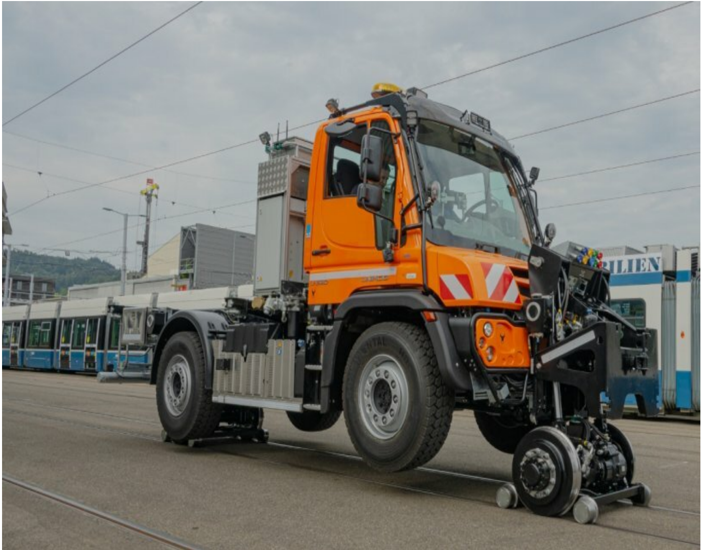
Unimog U 530 equipped as a multi-functional working machine with hydrostat drive for maintenance and servicing work at Verkehrsbetriebe Zürich (VBZ)
