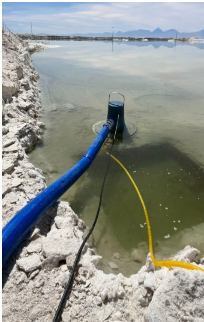
Atlas Copco WEDA electric dewatering pumps optimise lithium extraction process at Chilean mine
