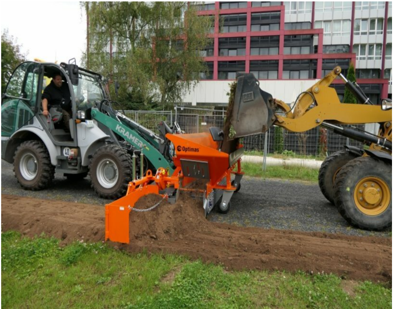
The Optimas material distribution bucket Finliner is filled with 1.4 m 3 by wheel loader or truck.
