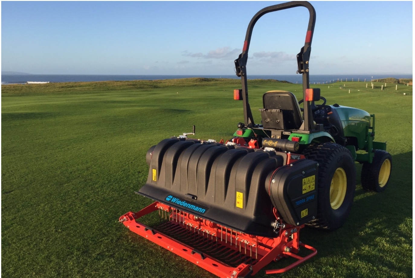
A Wiedenmann Terra Spike SL6 attached to a John Deere 2520.
