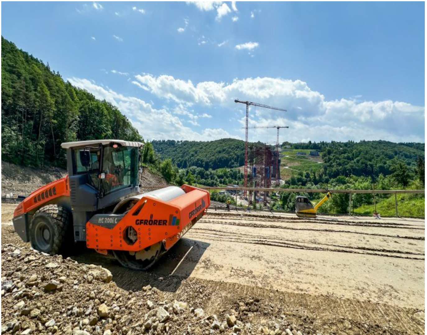
HC 200i C: High centrifugal forces of up to 350 kN, high torque for gradeability of up to 62%.
