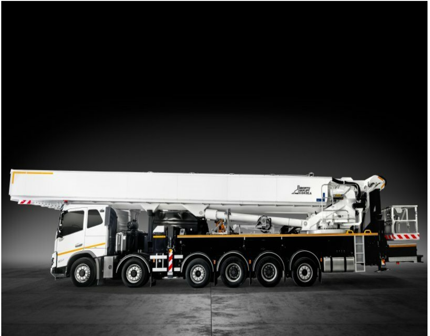
Bronto S104HLA mounted on a standard chassis
