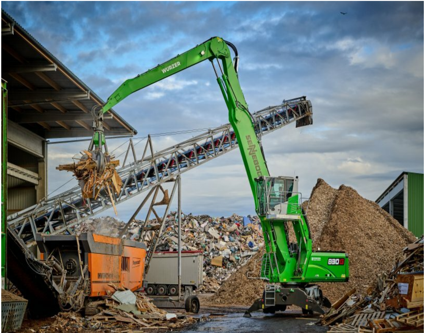
The green all-rounder feeds waste wood to a shredder at the Wurzer Umwelt site in Eitting.
