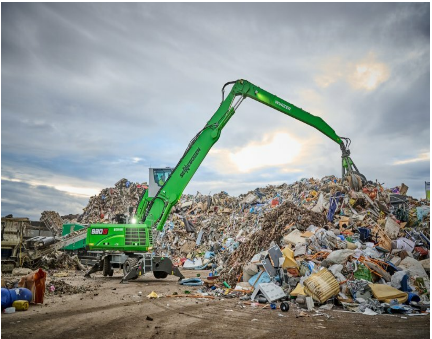
SENNEBOGEN 830 G: precise material handling with an 800 l polyp orange peel grab.
