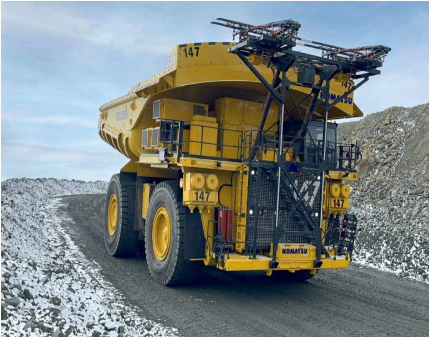
A Komatsu 930E diesel trolley PA truck at the Boliden Aitik Mine.
