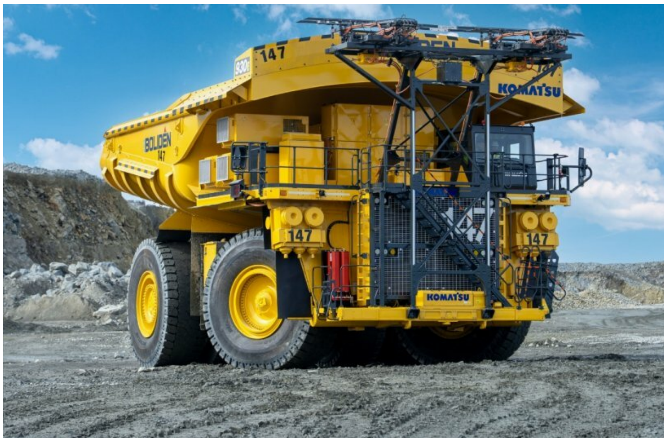
A Komatsu 930E diesel trolley PA truck at the Boliden Aitik Mine.
