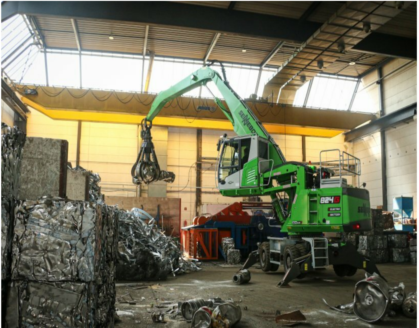
The integrated work area limitation protects against collisions with the roof in the hall.
