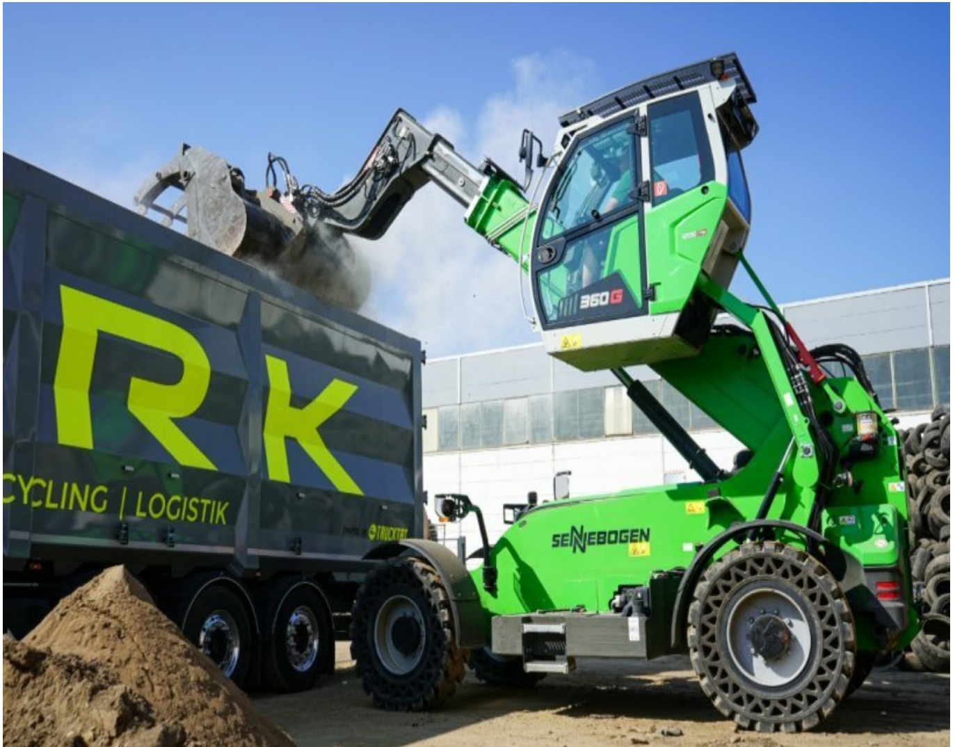
Compact on the move: The 360 G scores highly when loading in confined spaces.
