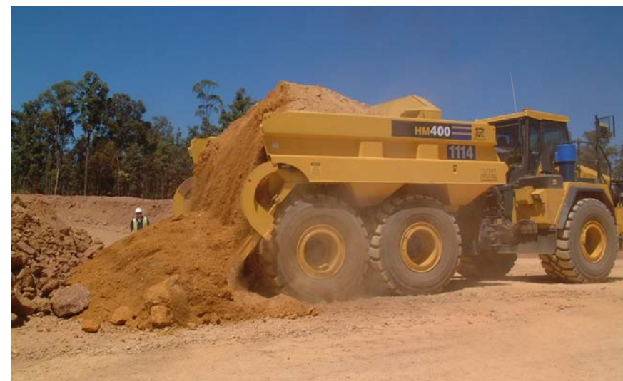
Without moving or raising the truck bed, the ejector blade of a Rear Eject Body pushes material toward the rear of the truck, while the tailgate lowers down and material is completely ejected. In eliminating the need to raise the body of the truck, Philippi-Hagenbuch Rear Eject Bodies allow for safely dumping materials while in motion and in the presence of overhead barriers.
