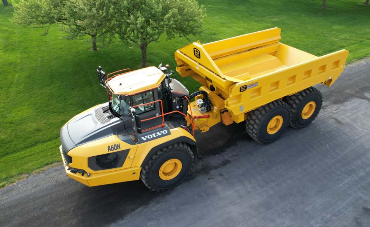
Philippi-Hagenbuch's patented line of Rear Eject Bodies offer the ideal solution for challenging hauling applications from general construction, road construction and sand/gravel to mine reclamation and underground hauling situations where overhead barriers inhibit traditional dump bodies.
