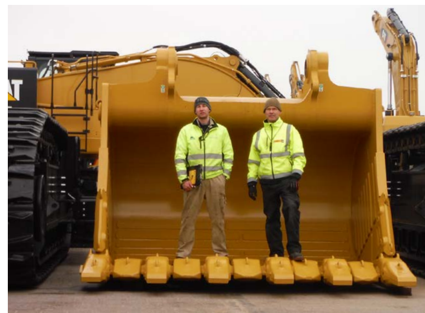
When the representatives of MEVAS were in the port of Antwerp for inspection of several motor graders they came across this Bucyrus excavator equipped with a 6 m³ bucket. It was disassembled for transport Image source: MEVAS
