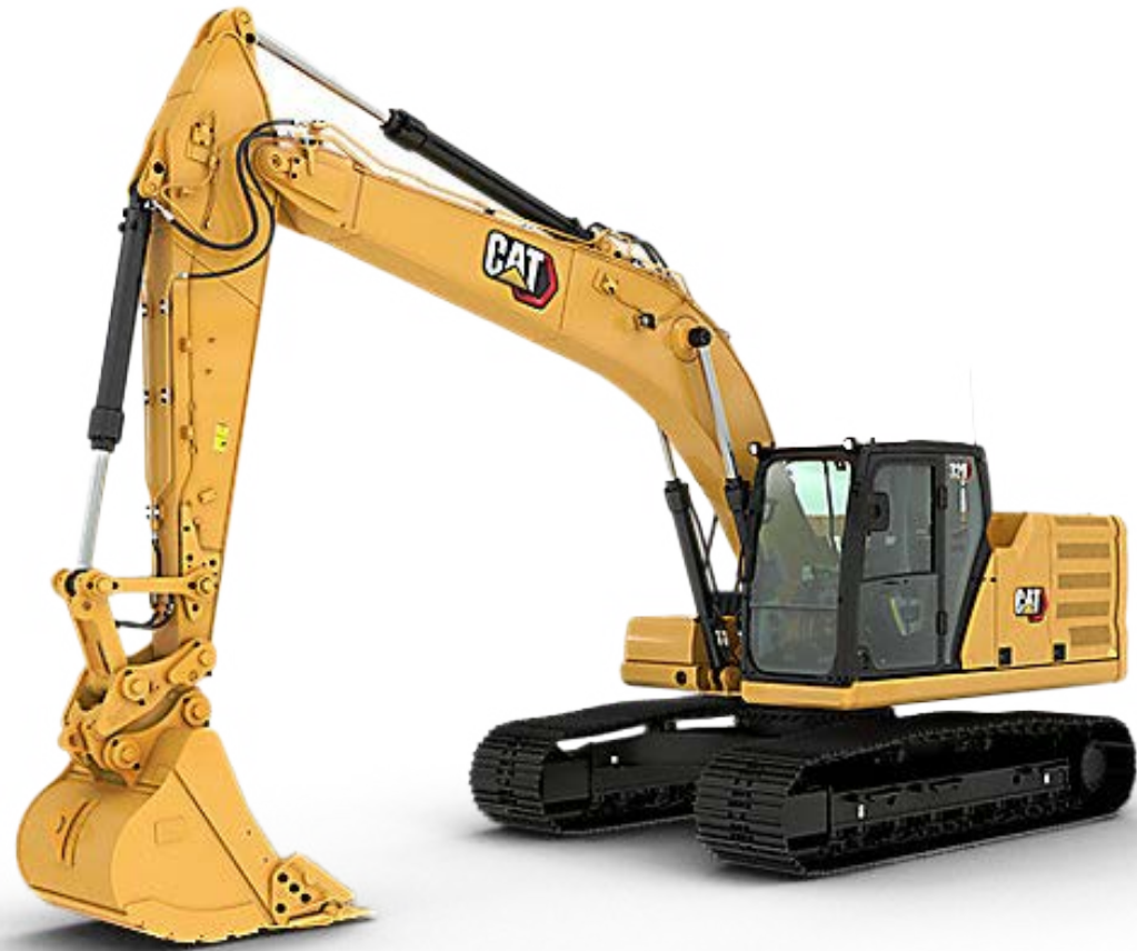
Caterpillar 320 crawler excavator Image source: Caterpillar
