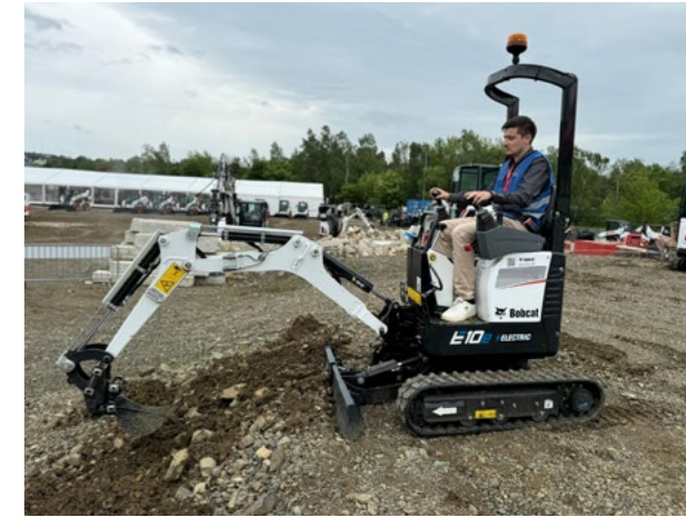
Patrik Eder operating the E10e mini excavator Image source: Doosan Bobcat EMEAzfg
