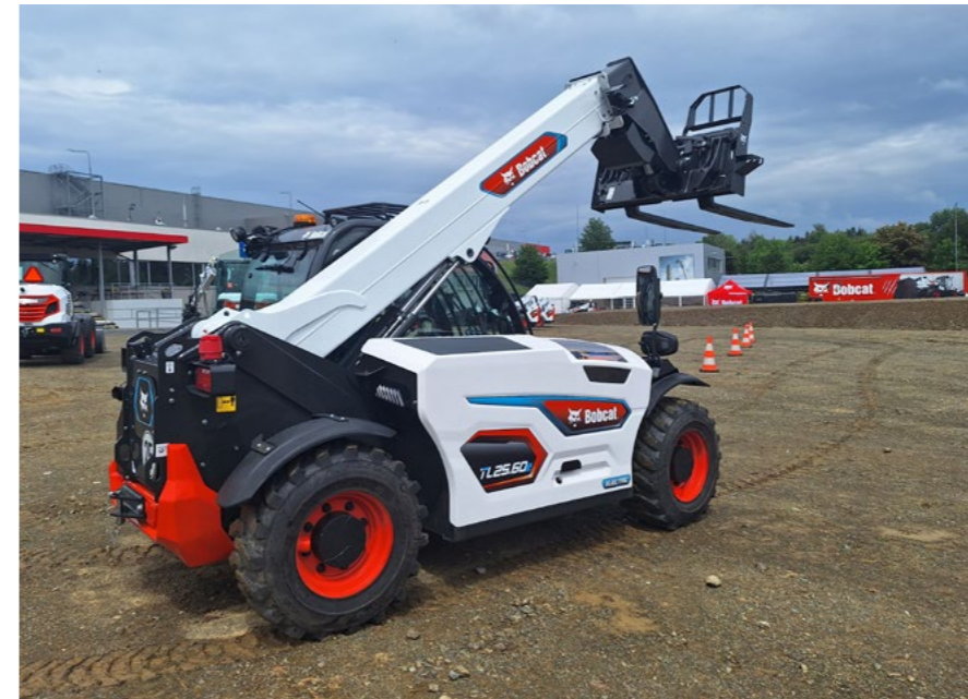
TL25.60e electric telehandler prototype Image source: Patrik Eder, LECTURA GmbH
