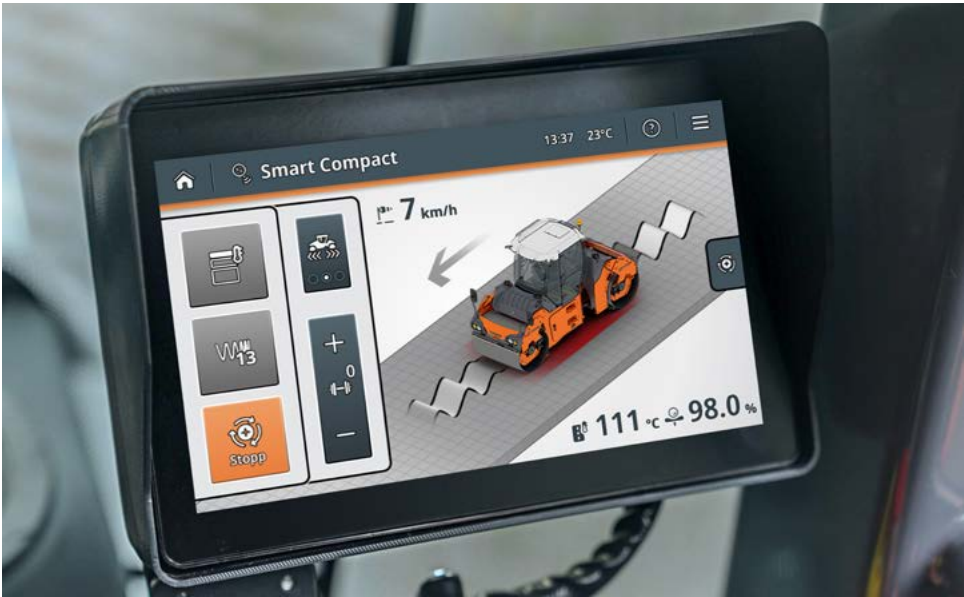
Integration of real-time density in Hamm Smart Compact: Automatic control of the compaction force and modes based on real-time density (shown in the bottom right of the display in %) offers construction companies decisive advantages when it comes to assessing compaction quality. Image source: Wirtgen Group
