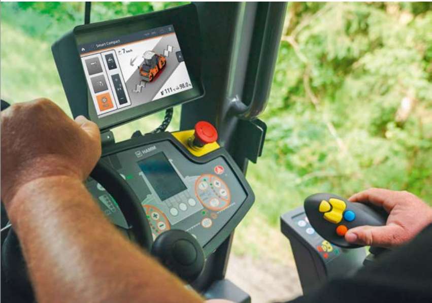
Easy to operate: Smart Compact Pro is intuitive to use thanks to the corresponding display. The highest compaction quality, which is achieved through automated compaction based on real-time density, is therefore possible even without years of experience. Image source: Wirtgen Group
