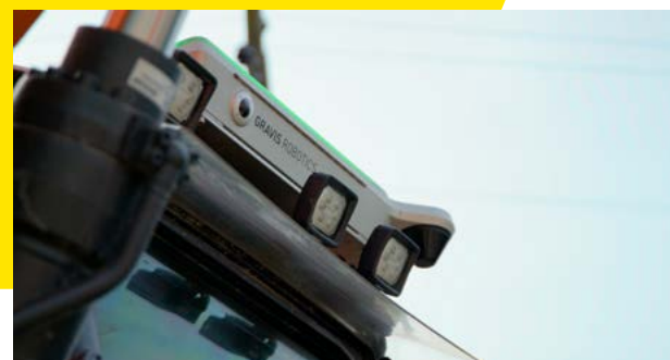
Detailed view: The Gravis Rack, a roof-mounted system, provides full LiDAR coverage for 3D scans of the surroundings. Image source: Gravis Robotics
